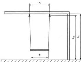
the maximum height of swing should be less than 60 cm and the minimum height from ground is 35 cm
